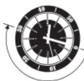
If your watch is equipped with a rotatable outer dial with one-minute graduations, this can be used in various ways to check elapsed time. For example if a diver has a 30-minute air supply, he can set the outer ring so that the triangle is in line with the minute hand when he submerges. The minute hand will then indicate on the outer ring the length of time that the diver has been under water.
