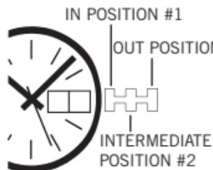
1. Pull out the setting crown to position #3. Move the hands forward by turning the crown. Observe the date as the hands move past 12 o'clock. When the date changes it is midnight on the watch. Set the hands to correct A.M. or P.M. time. Push the crown back in to position #1
